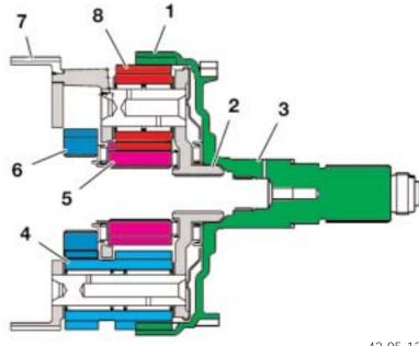
**Double Planetary Gear Train**
